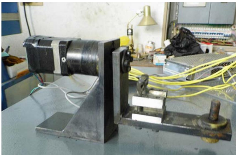
Figure. 4 Physical picture of the electric spark dressing device
