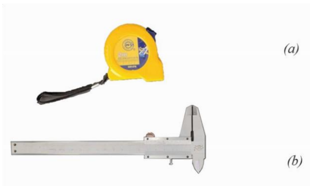
(a)- tape (b)- Vernier caliper Figure 8: Length measuring tool
