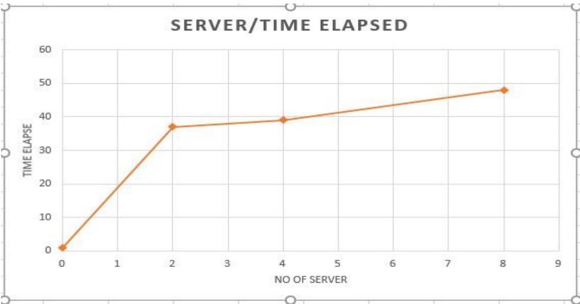
Figure 6: Server against time elapsed Figure 6 shows number of servers against the time it takes to complete a load balancing process. It is clear that, the number of servers also affects the time the system takes to balance or redistribute workload among cooperating nodes in the system.
