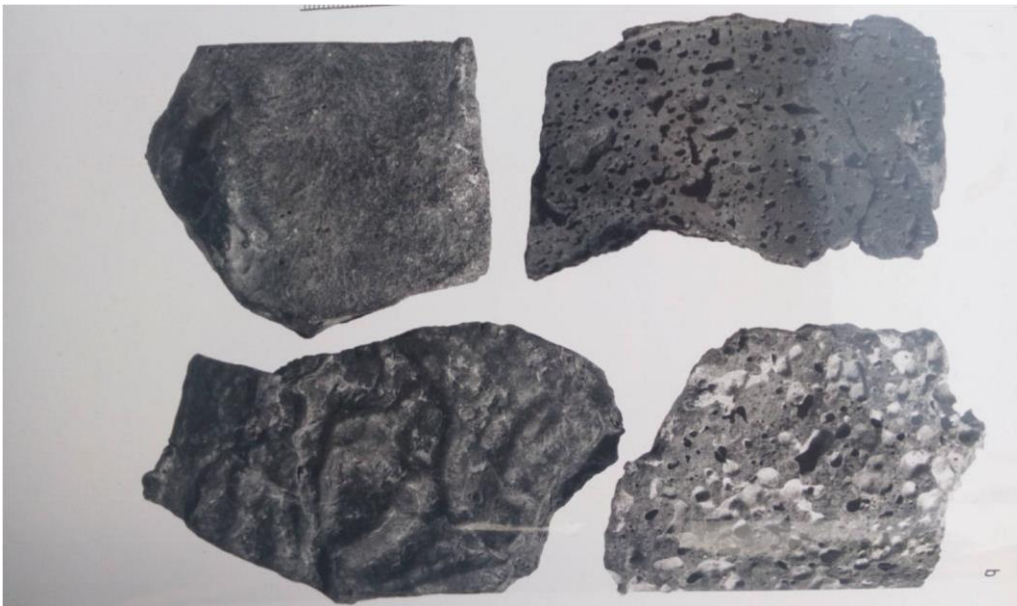
Figure 1. Photographs of typical DSC slag- (a) flat and smooth lower-face, (b) smooth, undulating lower-face both having tiny netlike cracks containing whitish infillings and coating; (c) showing rough, vesicular surface texture (deep pores) like a volcanic lava, and (d) also showing a very rough, vesicular surface (deep pores) texture with whitish lime infillings and coatings.
