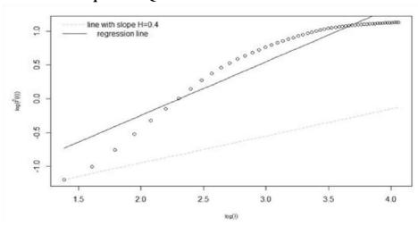
Figure 3.Plot Presenting the Scaling Properties of SDFA in -Scale for the Seismic Trace Signal of Explosion EX4.
