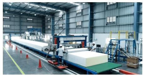
It specializes in transforming 30-meter-long foam blocks into various end products. Additionally, the facility features a well-organized curing area to ensure the thermal and dimensional stability of the foam products.
