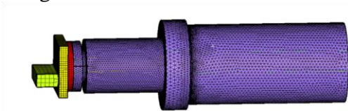
Figure 6: The whole model meshing
