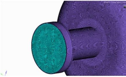
Figure 4: Model of the fluid meshing
