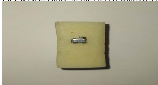
Fig. 5: Bracket bonded on the surface treated block ready for SBS testing.
