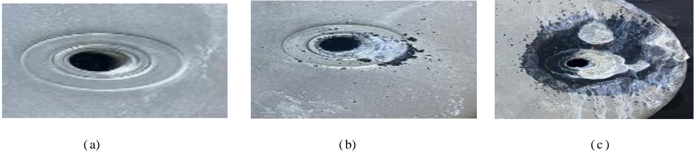
Figure 6. Appearance of electro galvanized specimen a) before salt fog test b) at 192 hours c) at 480 hours
